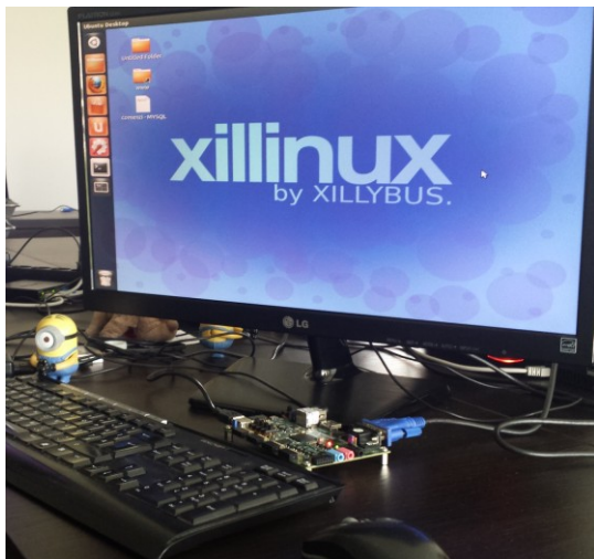
Fig. 6 Workstation with Zybo board used in tests (Zybo is based on Zynq 7000 SoC)
