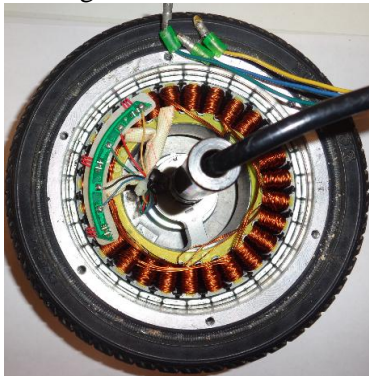
Fig. 2 The fabrication of the motor embedded in the wheel
