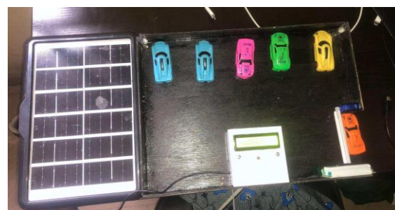
Fig. 4 Design Prototype of the automatic car park management system
